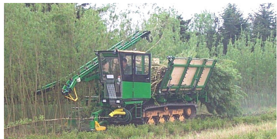
Whole stem SRC harvester, developed by NORDIC BIOMASS and Border Biofuels LTD.
