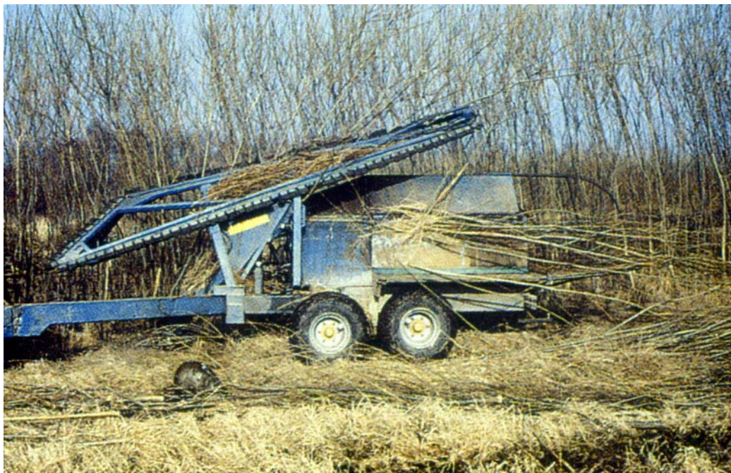
Figure 2. Tractor powered stick harvester suitable for small scale harvesting
